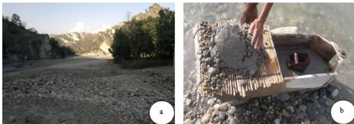
Figure 3: (a) Natrhal Khad, Chowki Choura, Akhnoor (b) Miner doing Sieving & Panning to collect gold flakes
