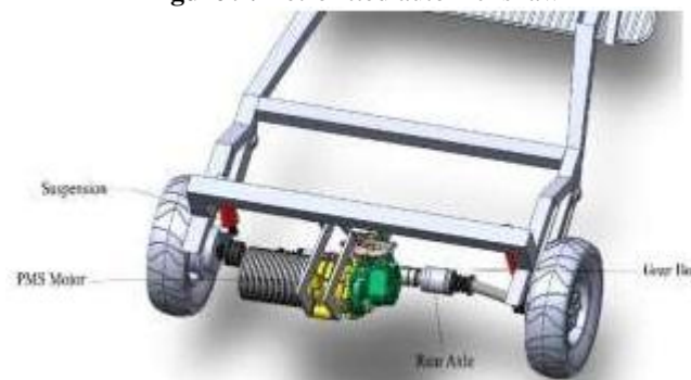
Figure 10: Assembly of components on chassis
