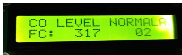
Figure 3: LCD DISPLAY (A) CO Level [Normal] and FC Date Monitoring
