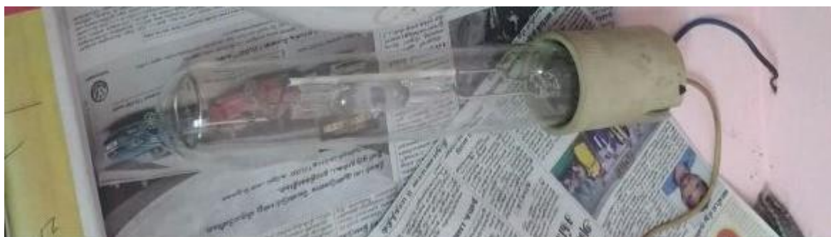
Figure 2 (b): Unshielded Metal Halide lamp
