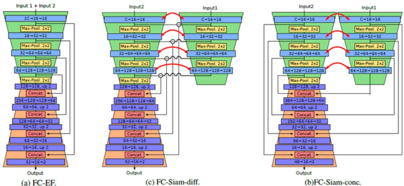
**Figure 3:** Schematics of the three proposed architectures for change detection. Block color legend: blue is convolution, yellow is max pooling, red is concatenation, purple is transpose convolution. Red arrows illustrate shared weights
