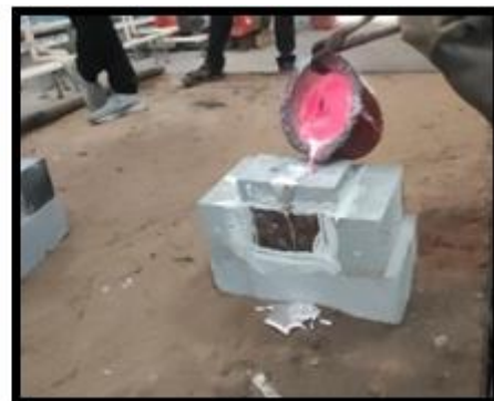
Figure 1: (a) Mold with chill plate, (b) side view of mold, (c) Resistance furnace, (d) pouring of the melt (molten composite)
