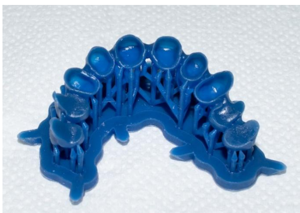
Figure 6: The 3D printed denture framework after the alcohol bath
