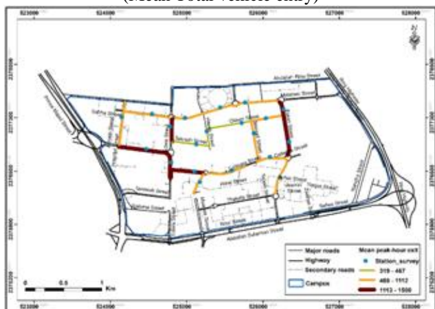
Figure 14: Map of traffic conditions in street segments (Mean Peak hour vehicle exit)
