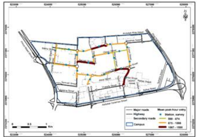
Figure 12: Map of traffic conditions in street segments (Mean Peak hour vehicle entry)
