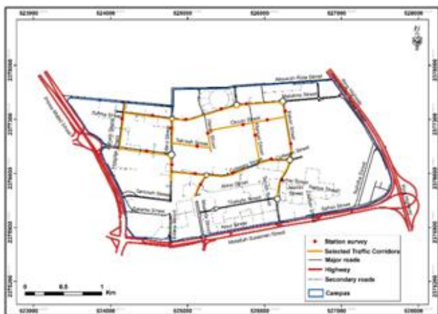
Figure 11: Survey station on selected traffic corridors in King Abdulaziz University
