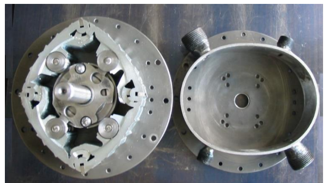
Figure 1: Quasiturbine Model QT-SC (without carriage) with 4 Blades Rotor, the Contour Seals, wheel-bearing Blade support, and a Shaft Differential [15]. Stator in Expander Mode with intakes and large exhaust ports, including side covers.
