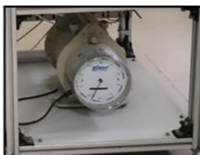
Figure 13: Gas Flow Meter
