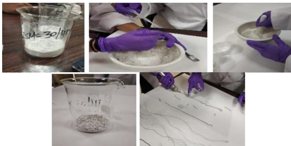
Figure 4: Synthesis of Extruded ZSM-5
