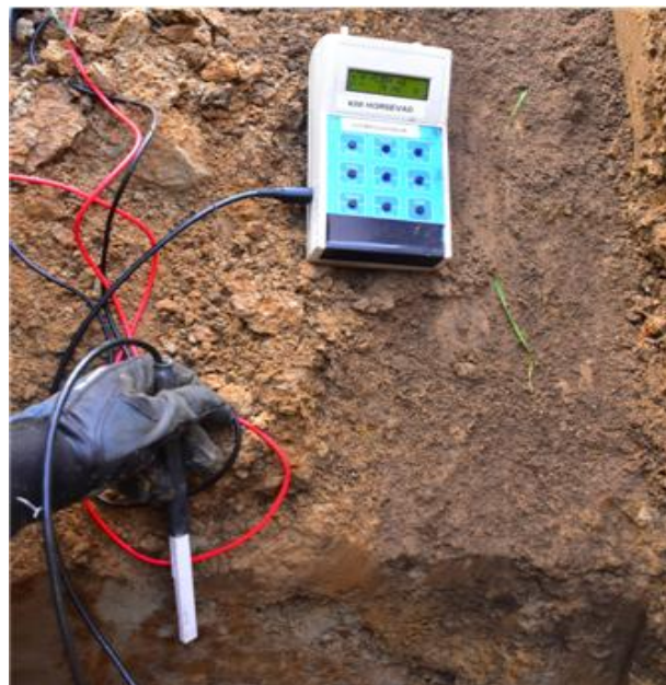
Figure 1: Measurement of magnetic field intensity directly upon an electrically conductive layer of ocher in 2, 7 meters depth. A maximum reading of 135, 4 \mu T (1354 mG) was recorded. Image from (8)
