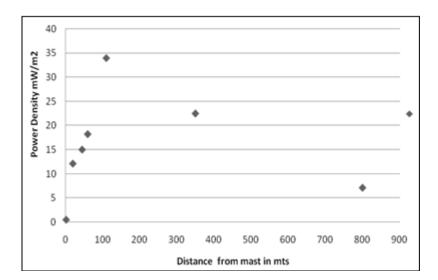
The graph shows that distance from transmitting antenna is important factor in residential areas. Maximum density was observed between 100 to 140 mts. This means that the people residing within this radar have highest exposure to the radiation which may result in serious consequences on human health and environment as a whole.
