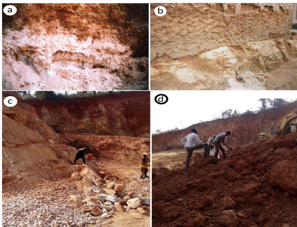
Figure 4: (a) A photograph showing exposure of a Kaolin deposit in Ijero-Ekiti, (b) Kaolin deposit formed in-situ by chemical decay of a pegmatite forming a sub-base to a building in Odo-Owa, near Ipoti-Ekiti, (c) Resizing massive quartzite into chips for construction through manual labour in Ado-Ekiti, (d) harvesting laterites and lateritic soils as engineering fill material along Secretariat (Bank) road, Ado-Ekiti.
