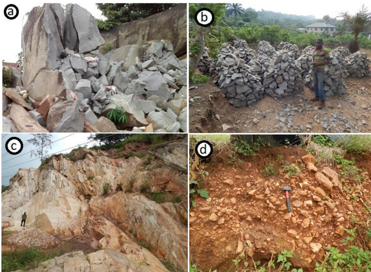
Figure 3: (a) a freshly blasted microgranite to make space for a building in Okeyimi area of Ado-Ekiti (b) The rock chips are sorted according to sizes desirable for sub-base materials in construction (c) Quartzite harvested from massive quartzite awaiting buyers between Itawure/Ita-Ido junctions near Oke-Mesi area of the State, (d) natural gravel deposit exposed beside a quartz rubble mining site of a major quartzite outcrop in Ajebandele area of Ado-Ekiti.
