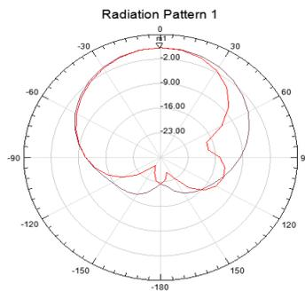
Figure 4: V-slot MSA radiation pattern
