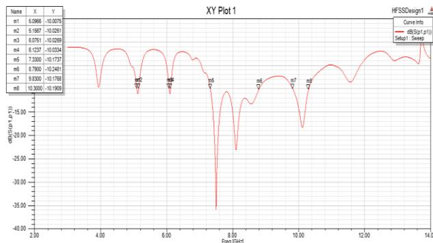
Figure 6: Return loss against frequency of 5SMSA
