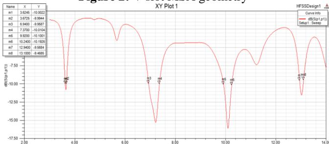
Figure 3: Return loss vs. frequency of V slot MSA
