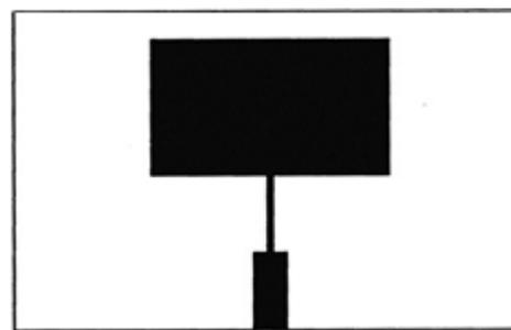
Figure 1(a): Conventional Microstrip Antenna
