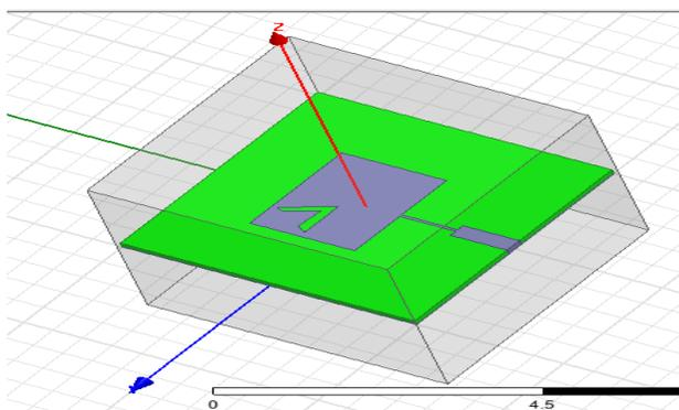
Figure 2: V slot MSA geometry
