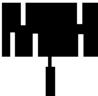
Figure 1(c): Five vertical slot Microstrip Antenna
