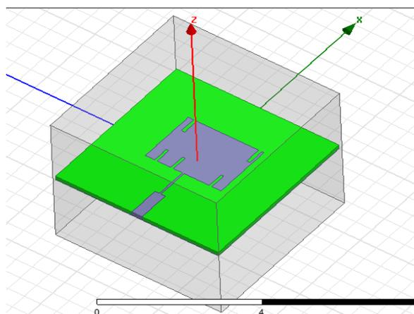
Figure 5: Geometry view of 5SMSA
