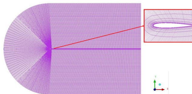
Figure 2: Structured mesh of the computational domain
