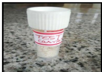
Figure 2: shows the chitin-chitosan carrier obtained by adsorption process
