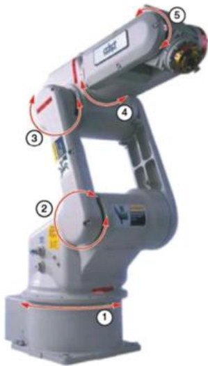
Figure 4: A robot with revolute configuration. It has 5 arm joints
