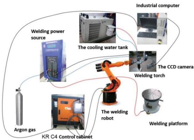
Figure 2: Robotic TIG Welding
