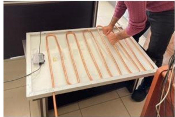
Figure 2.2: Placing water pipes at the bottom of the PV panel
