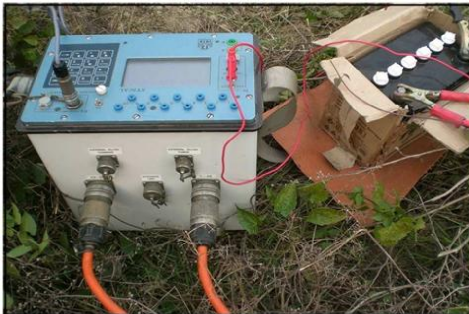
Figure 4.11: IRIS make SYSCAL Pro – 96 Field equipment used for the survey
