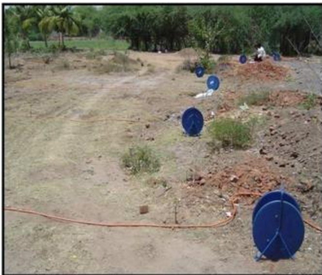
Figure 4.4: Multi-electrode winch set-up
