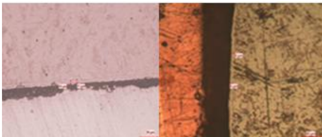
Figure 2: Microstructures of specimens undergone Nitrocarburising without preoxidation a) 2 hr duration of exposure b) 4 hr duration of exposure
