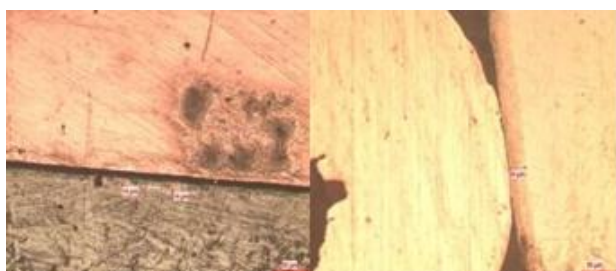
Figure 4: Microstructures of specimens undergone Nitrocarburising with \text{CO}_2 as preoxidant a) 2 hr duration of exposure b) 4 hr duration of exposure.
