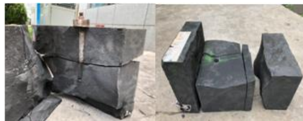
Figure 12: Cracking and Crushing Effects of Core E
