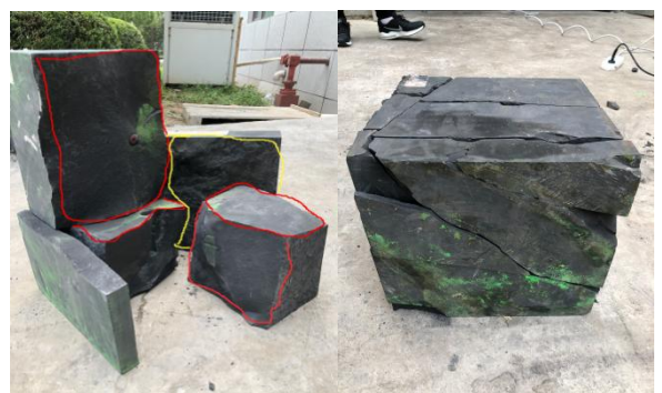
Figure 6: Cracking and Crushing Effects of Core B
