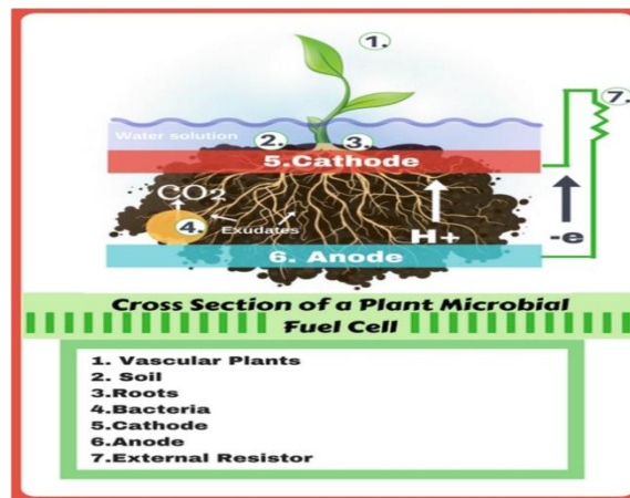
Figure 2: Cross section of a PMFC
