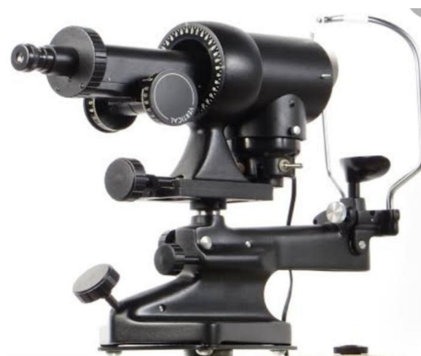
Figure 2: Bausch and Lomb Manual Keratometer
