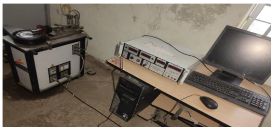
Figure 2: DUCOM-TR20 LE pin-on-disk set up
