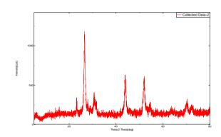
Power diffraction of the samples were done using coupled  $2 \Theta/\Theta$  scan type in continuous scan mode from  $2 \Theta$  angle of 3.000 ° to 80.002 °, sample rotation 15.0001 per minute, using copper anode, wavelength for display at 1.54060 A using Lynx eye detector and crystallinity from 3.000 to 80.002.
