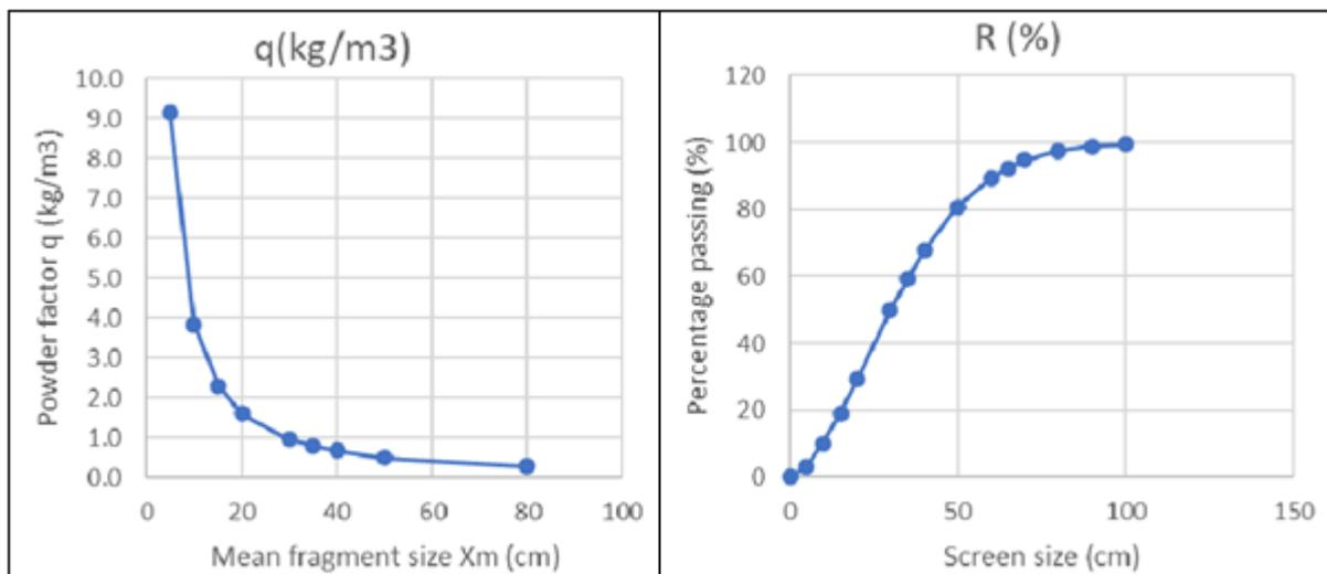
(a) Mean fragment size for 114 and 115 mm. (b) Percentage passing for 114 and 115 mm
