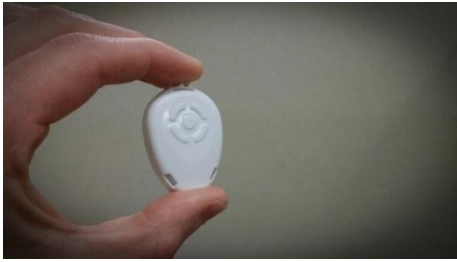
Figure: A WISER Locator tracker tag used for UWB asset tracking
