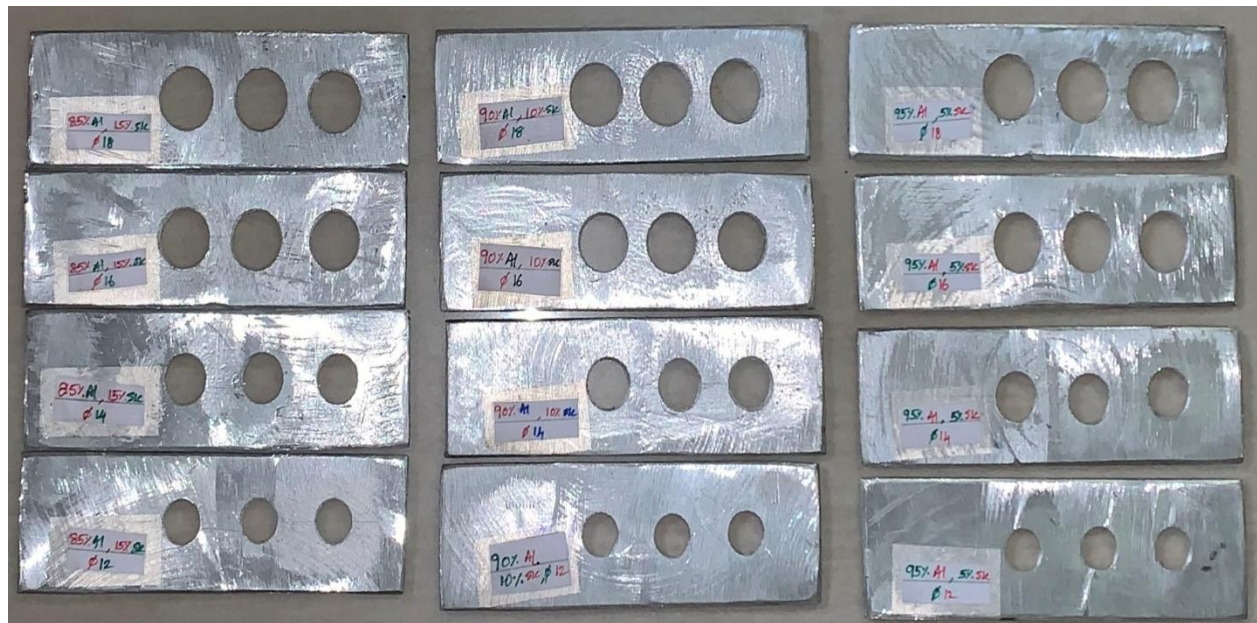
Figure 4 (b): Types of fins (a) Perforated 85% Al-15% SiC fins (b) Perforated 90% Al-10% SiC fins (c) Perforated 95% Al-5% SiC fins. In above three cases perforations vary from 12mm - 18mm diameter.
