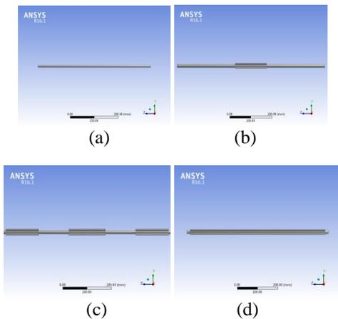
**Figure 1.4:** finite element model of pipeline (a) without stiffeners (b) stiffener of length 150 mm (c) stiffener of length 420 mm (d) stiffener of length 670 mm
