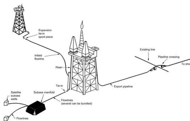
Figure 1.1: Subsea pipelines
