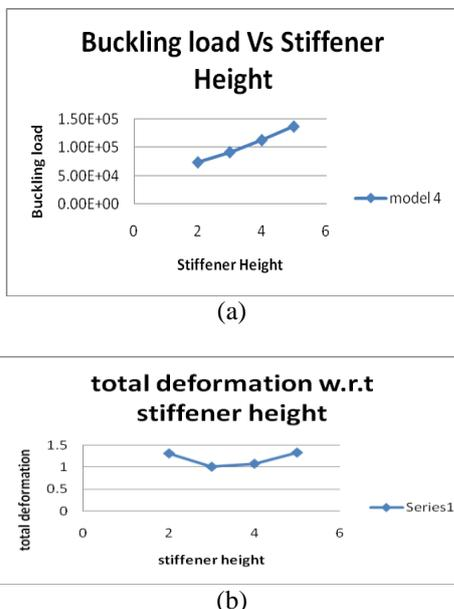
Figure 1.9: Graph showing (a) buckling load vs. height (b) total deformation Vs stiffener height
