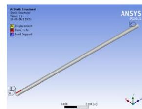
**Figure 1.7:** boundary condition of (a) without stiffeners
