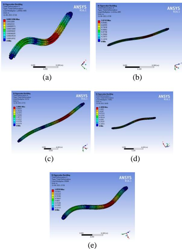
Figure 1.8: Contour showing buckling of pipeline of models (w. r. t height) of (a) stiffener of length 670 mm with height 5 mm (b) stiffener of length 670 mm with height 4 mm (c) stiffener of length 670 mm with height 3 mm (d) stiffener of length 670 mm with height 2 mm
