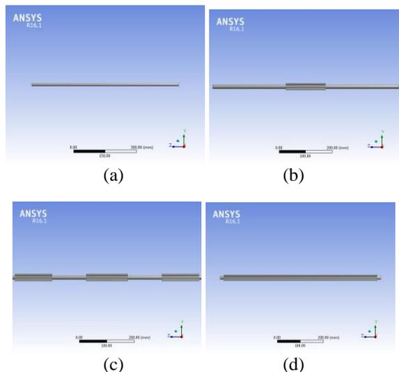
**Figure 1.5:** finite element model of pipeline (a) without stiffeners (b) stiffener of length 150 mm (c) stiffener of length 420 mm (d) stiffener of length 670 mm
