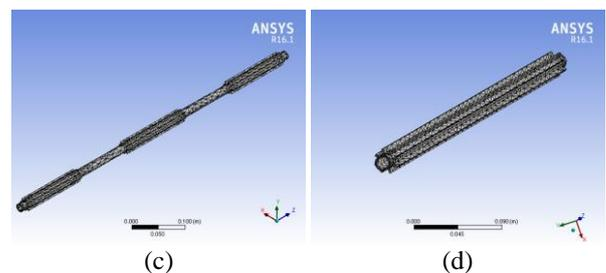
**Figure 1.6:** Mesh models of (a) without stiffeners (b) stiffener of length 150 mm (c) stiffener of length 420 mm (d) stiffener of length 670 mm
