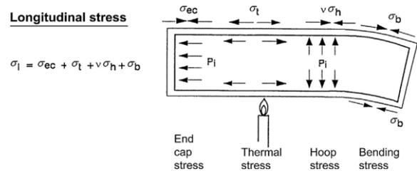
Figure 1.3: Longitudinal stress of pipeline
