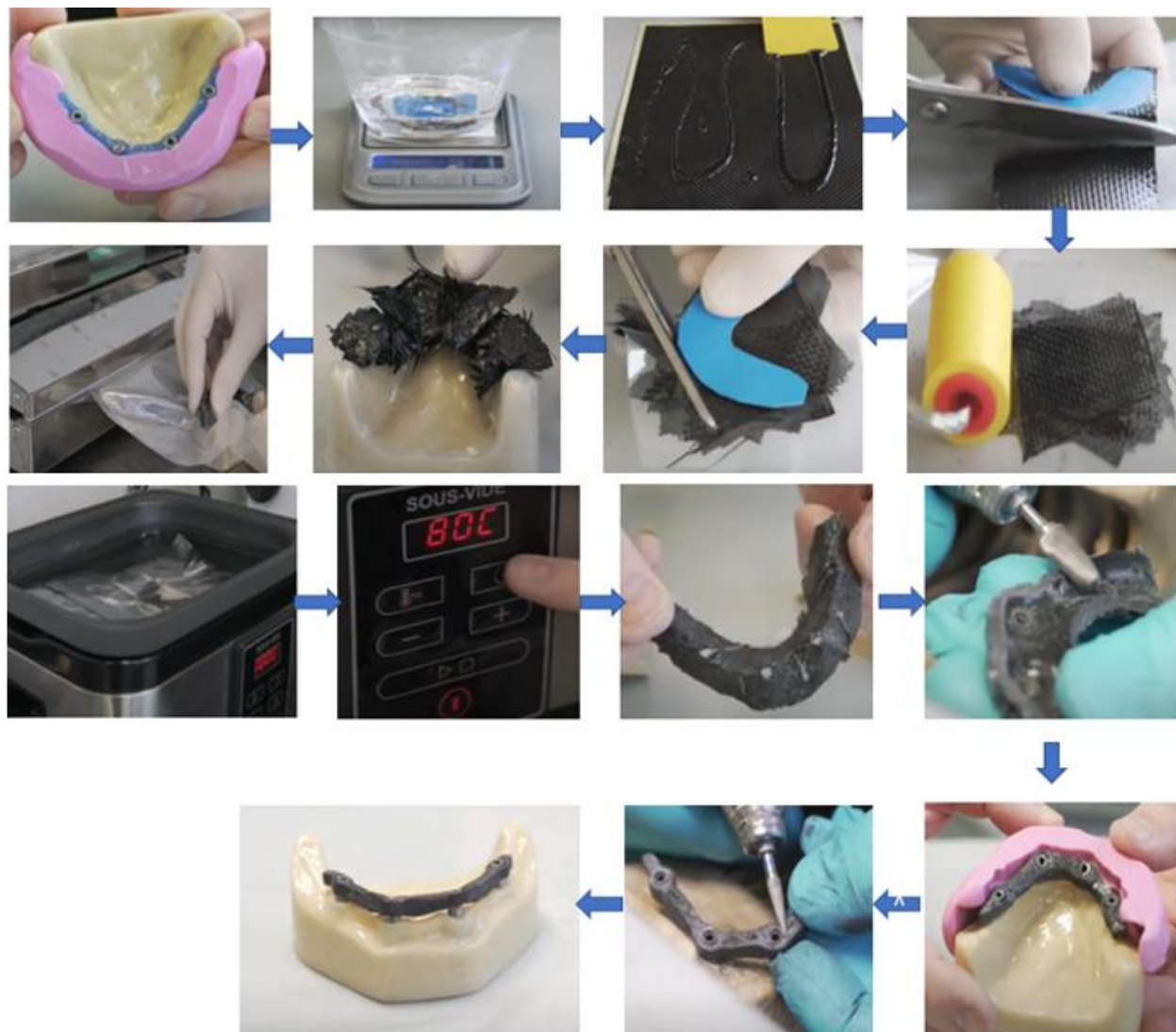
Figure 9: Superimposing and pressure moulding technique
