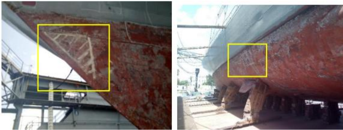
Figure 1: Acquisition of samples of the 37-year-old ship; front and middle area (samples S1 and S2)
