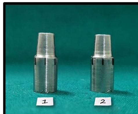
Figure 2: Stainless steel dies mounted on a metal jig
