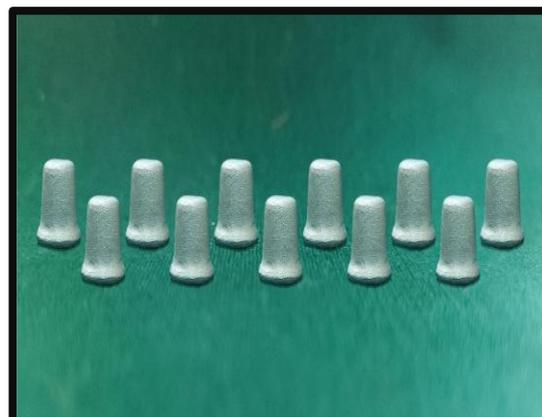
**Figure 12:** 11 samples fabricated by DMLS technique with deep chamfer margin.
