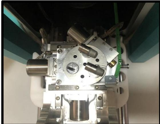
Figure 13: Mounting of samples on the platform of SEM.
