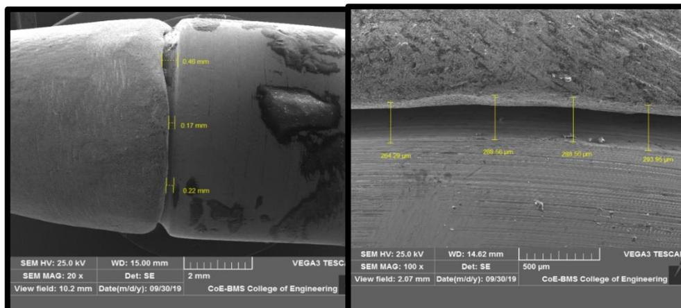
Figure 15: Determination of marginal fit.
