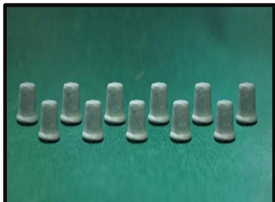
**Figure 7:** 11 samples fabricated by conventional technique with deep chamfer margin
