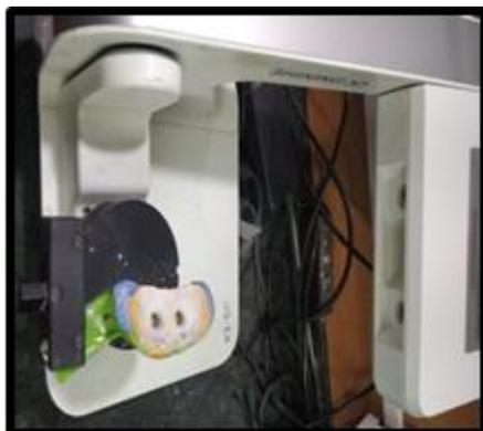
**Figure 8:** Putty wash impression of both the stainless steel dies being scanned
