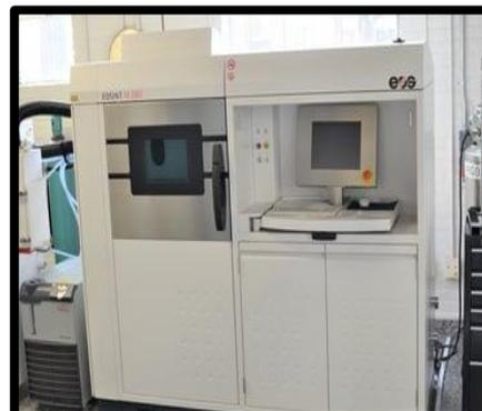
**Figure 10:** Direct Metal Laser Sintering (DMLS) 3D printing machine (EOS, Germany).
