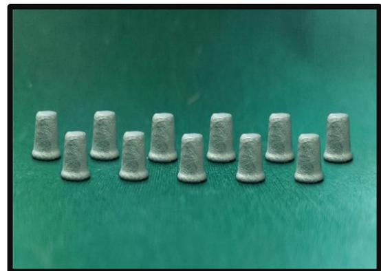
**Figure 6:** 11 samples fabricated by conventional technique with chamfer margin.
