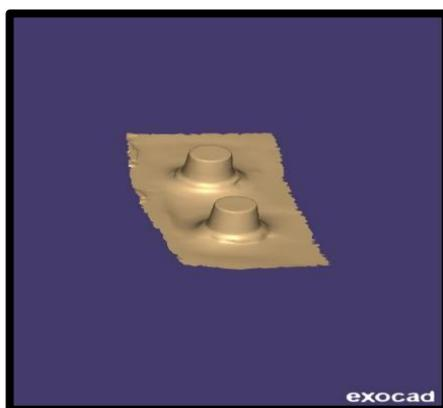
**Figure 9:** STL file of the scanned impression of two metal dies
