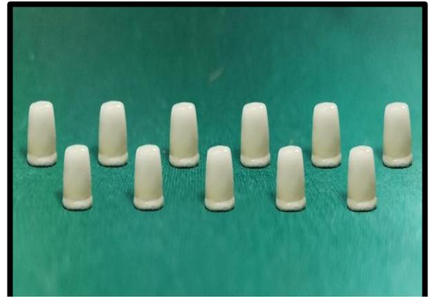
Figure 14: ceramic build - up & porcelain glazing done for the samples
