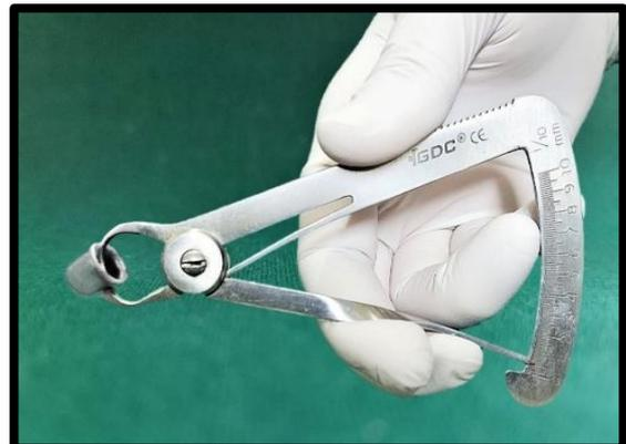
**Figure 5:** Verification for 0.5mm thickness of the sample using a metal gauge.
