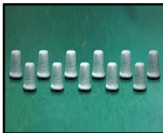
**Figure 11:** 11 samples fabricated by DMLS technique with chamfer margin
