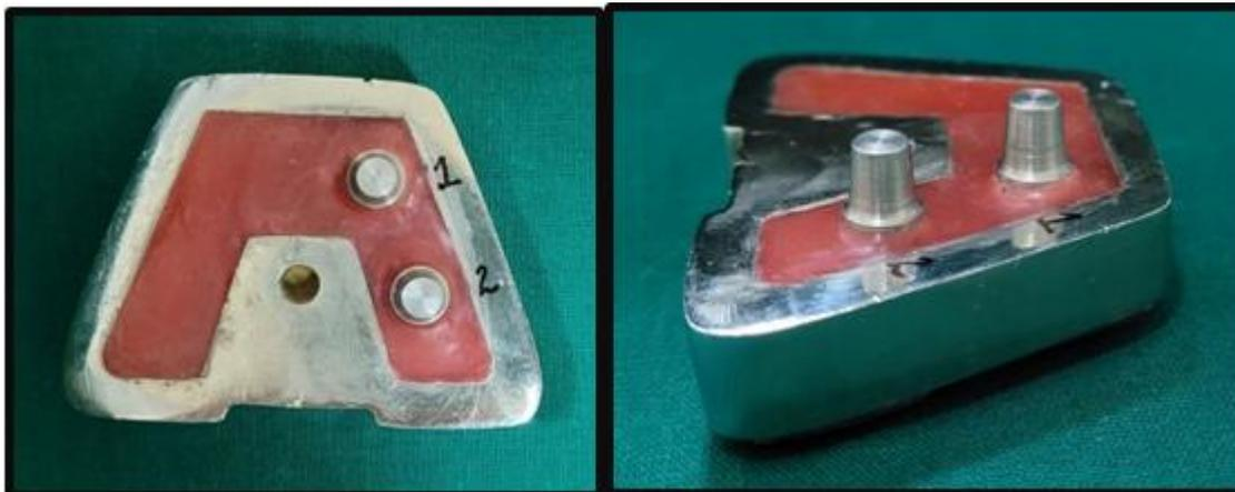
Figure 1: Stainless steel dies mounted on a metal jig
