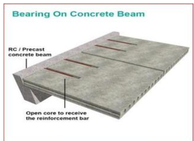
Fig 1.2 : Voided slab Connection with Concrete Beam
