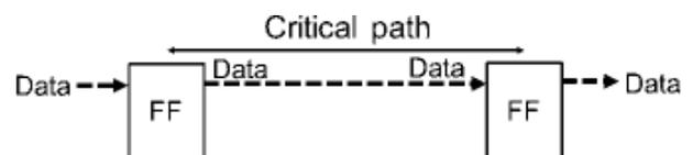
Figure 1: (a) Critical path of a sequential circuit
