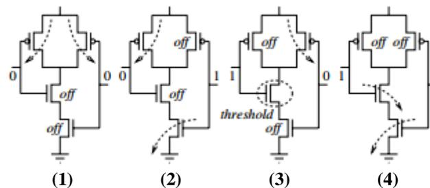
Figure 7: States of 2 input NAND gate
