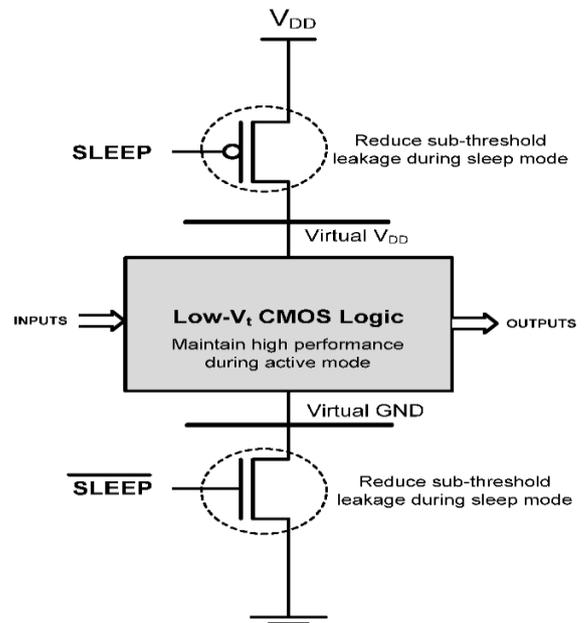
Figure 2: General MTCMOS circuit architecture
