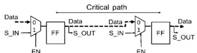
Figure 1: (b) Critical path after scan insertion
