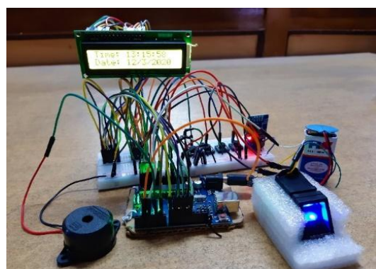
Figure 6: The experimental setup of “Automated Biometric Attendance Recorder”
