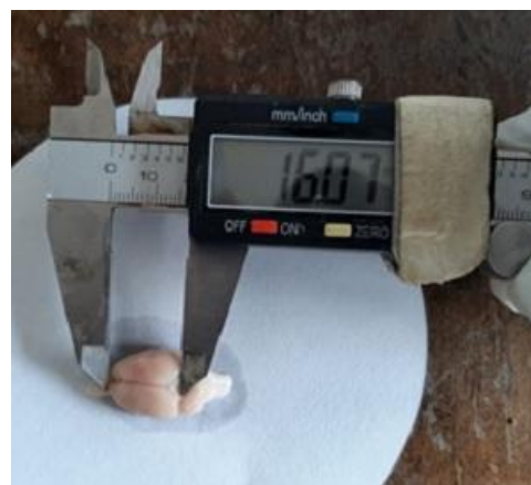
Figure 1: Method of measurement of the antero-posterior diameter of the rat brain to the nearest 0.01mm
