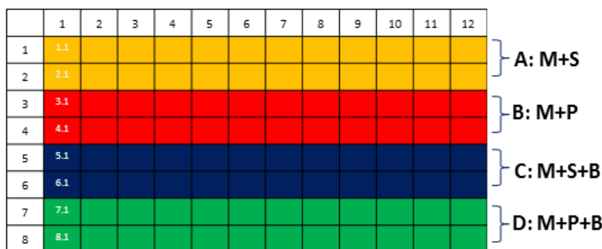
Figure 1: Layout microplate 96 well. M: media, S: sample, P: solvent, B: bacteria. (A) Media and samples. (B) Media and solvents. (C) Media, samples, and bacteria. (D) Media, solvents, and bacteria
