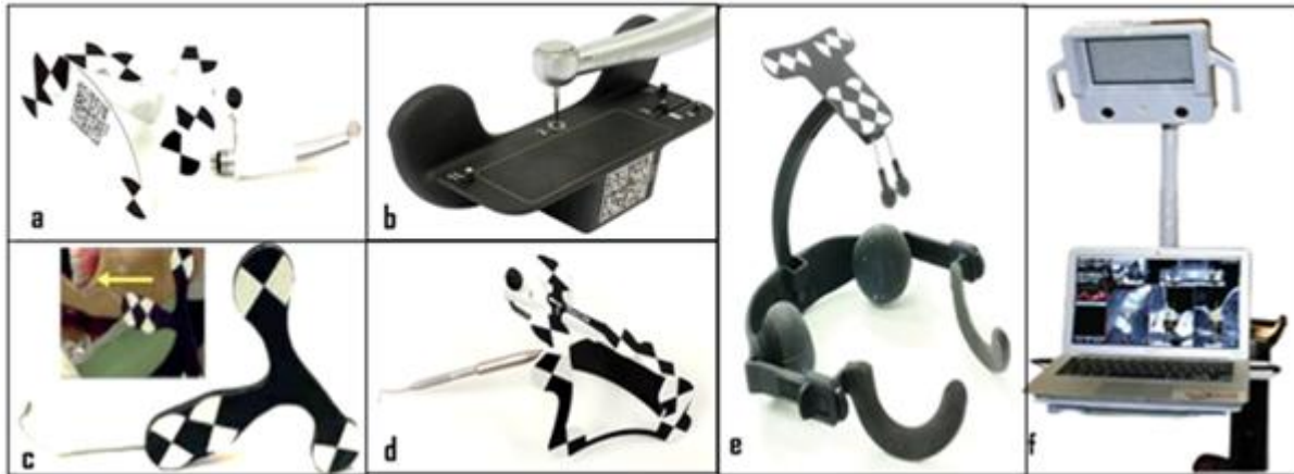
Figure 1: (a) Drill Tag mounted on handpiece, (b) Drill Calibrator calibrating the handpiece bur, (c) Jaw Tag with attachment clip, (d) Jaw Tracker for trace registration, (e) Head Tag for maxillary arch, (f) Stereoscopic motion sensing cameras with light present overhead with computer displaying the position through dynamic navigation software.
