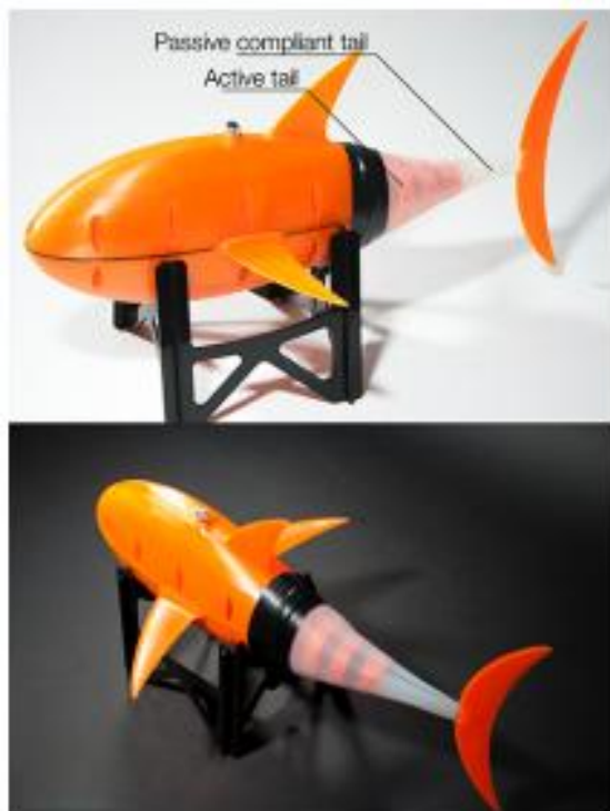
Figure 6 : Design of Robotic fish
