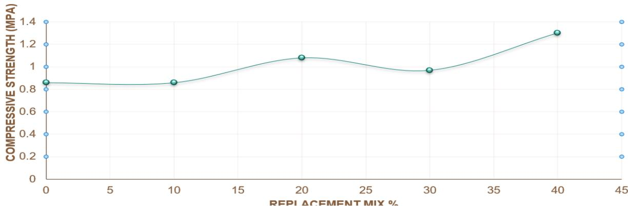
Graph 2: Compressive Strength at 100°C Steam Curing for 12 hours vs Replacement mix
