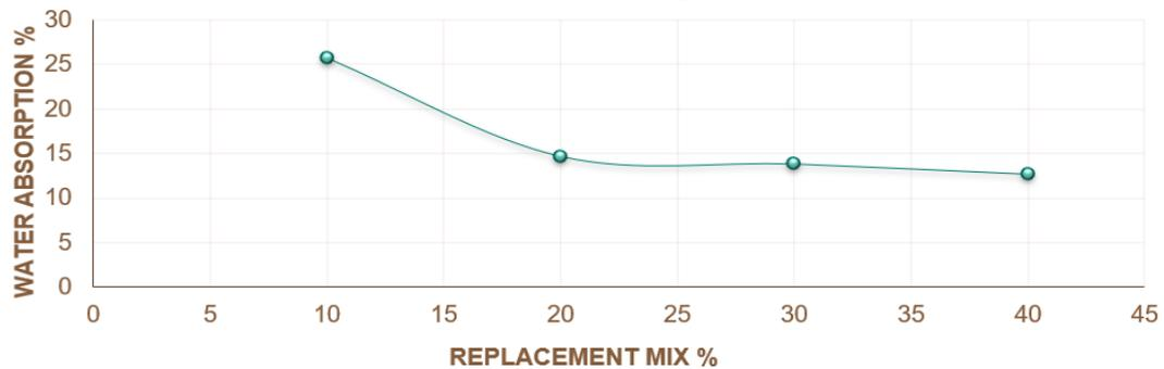
**Graph 4:** Water absorption % vs Replacement mix % (for 12hrs Steam Curing)
