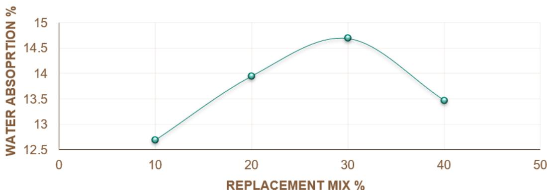
Graph 3: Water absorption % vs Replacement mix % (for 6 hours Steam Curing)
