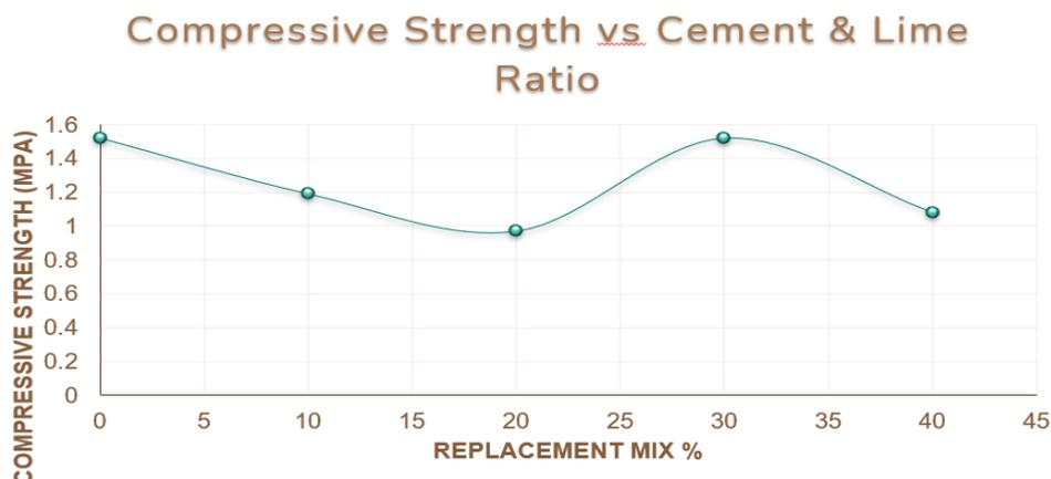
**Graph 1:** Compressive Strength at 100°C Steam Curing for 6 hours vs Replacement mix %
