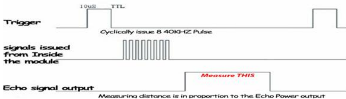
Figure 3: Timing Diagram for ultrasonic sensor
