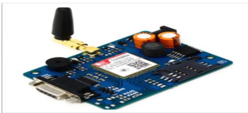
Figure 3: GSM module with antenna and serial interface port. Source-Google images
