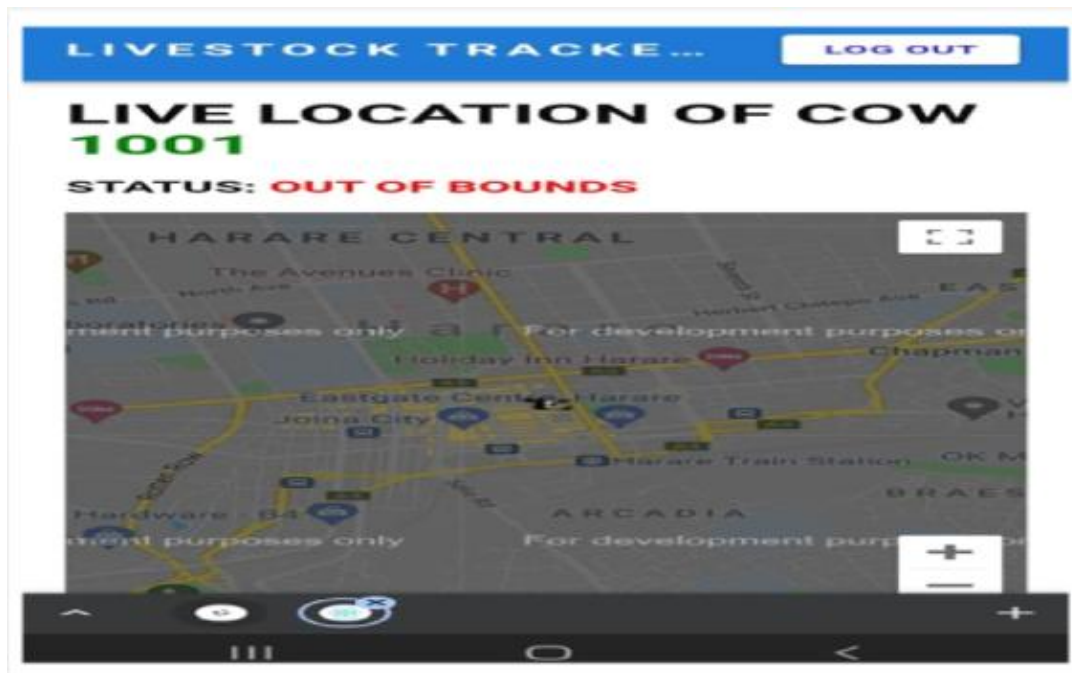
Figure 10: View showing an animal that has breached the perimeter 'geofence'
