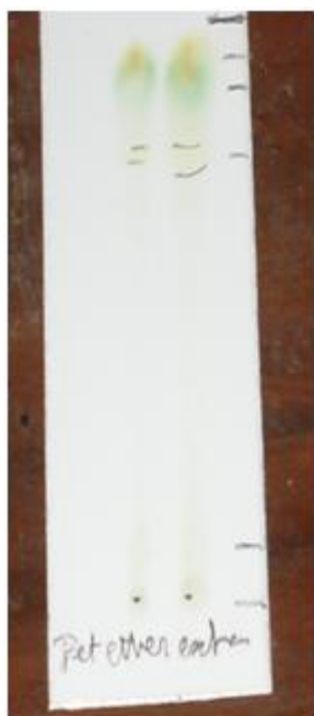
Figure 5.1: TLC profile of the pet. ether extract of P. guajava leaf. Solvent system: benzene: chloroform: ethyl acetate (4: 3: 3). Rf values: 0.10, 0.74, 0.87, 0.93.
