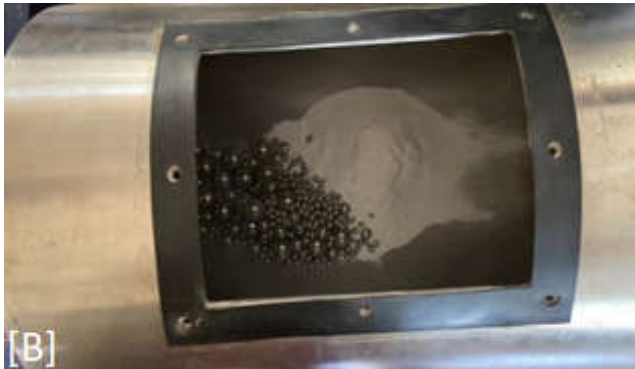
[B] Stainless steel balls used to dry mill
