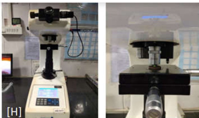
[H] Vickers microhardness test
