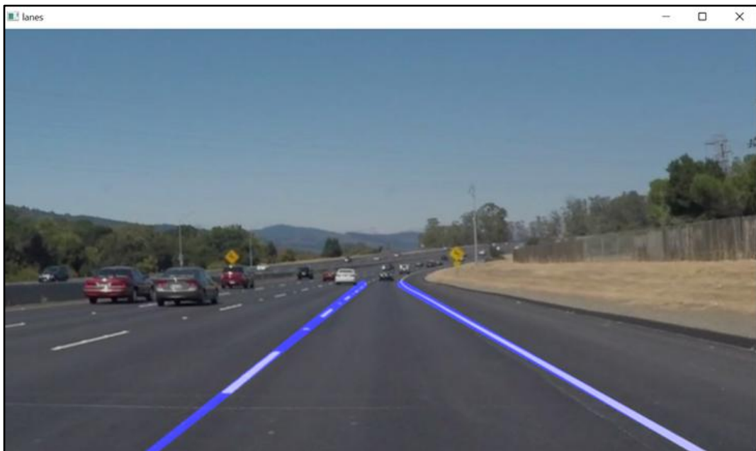
Figure 5: Final Output of Lane Detection
