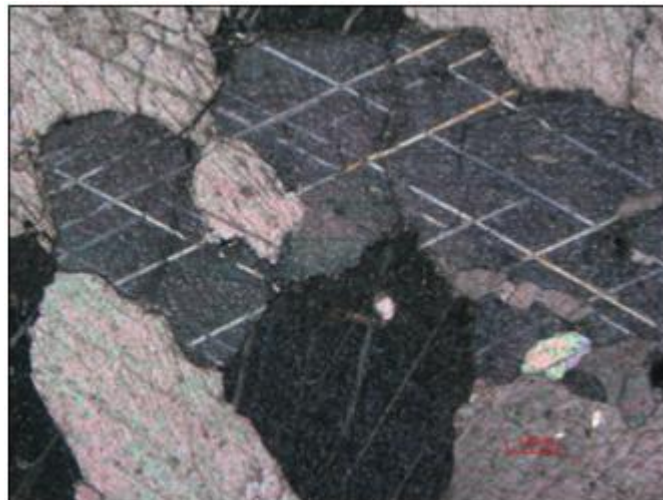
Figure 9: Microphotographs of dolomite grains showing well marked rhombohedral cleavages and twinning.
