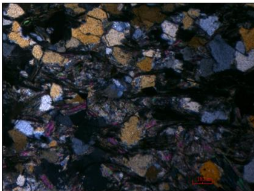
Figure 5: Microphotographs showing quartz, biotite and Muscovite minerals in micaceous quartzite rock.
