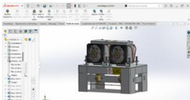
Figure 10: 3D modeling of the thermoelectric generator
