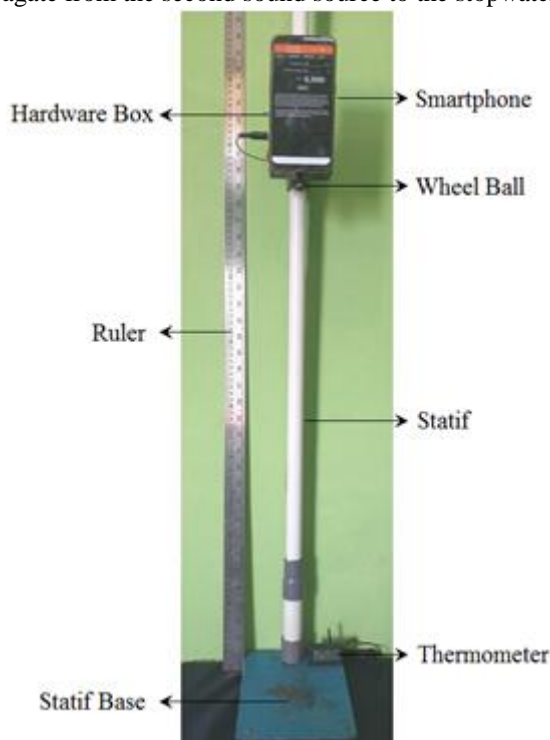
Figure 2: Experimental setup to determine the speed of sound in air
