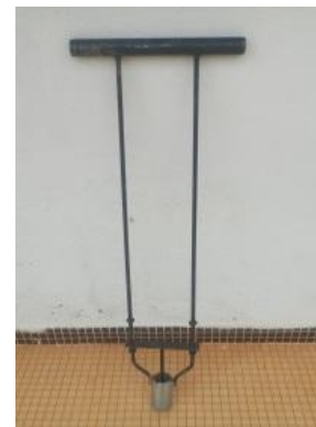
A tool for making nutriblocs from soil - based substrate. In the absence of an established term, it can be called "cylindroir".
