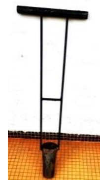
A tool that can be called a planter, allowing to make the holes in which the plants obtained on nutriblocs are placed.
