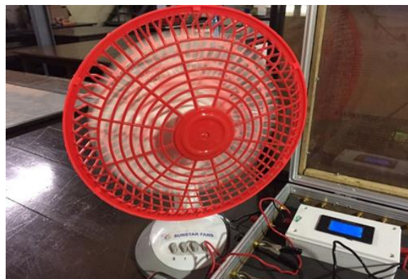
18 W 12 V DC Fan Running on 12 V Solar Battery
